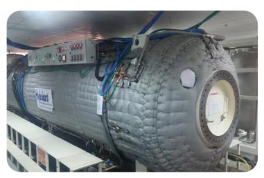
Hyperbaric and decompression / Therapeutic chamber for emergency - Chamber B (diam. 2200  $\times$  7000) - rated 20 bars -
